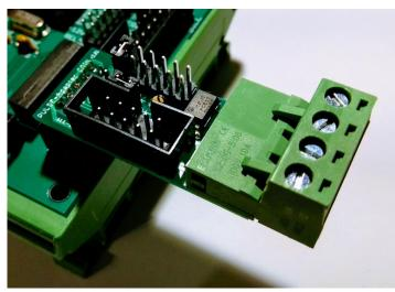
The PULSE-Adapter [Coin] is simply plugged into the 10 pin coin plug on the host board.
