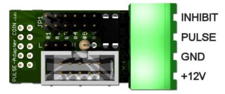
The PULSE-Adapter COIN has a 10 pin connector that fits to default coin plugs, and offers again a 10 pin coin plug to plug in the originally coin acceptor cable, so you do not lose the coin acceptor connector. By a jumper it is possible to select the coin channel, on which the external credit signal from the cashless system is transferred to. The external cash device can be controlled via INHIBIT of the coin plug, too.
