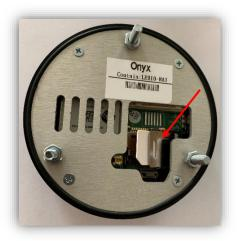
Step 2: Lock SIM card in place by pushing the cradle down onto the main board. Slip the silver clutch up to lock the card in place.
