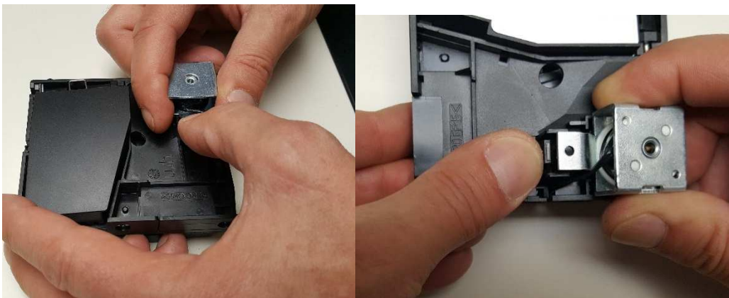
Fig. 6 Removing the solenoid from the selector EMP 800 v7 and 800 v6.
