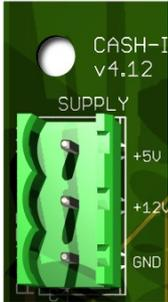
The power supply is connected to terminal plug X1.
