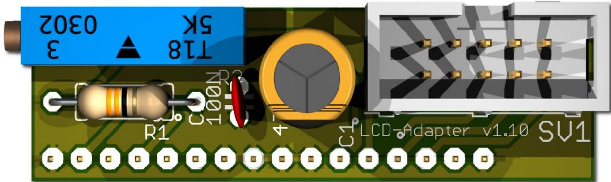
Depends on the used LCD display, the adapter has to be mounted on the left or right side. Some displays have the power pins on the left side others on the right side! Hint: since version 1.10 the LCD-Adapter only
