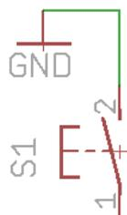
We want GROUND to every Pin, so simply wire the switch with GROUND!
