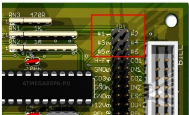
The #1 - #6 pins are located on the CASH-Interface2, JP1 pin header.
