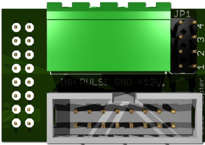
The PULSE-Adapter BILL has a 16 pin connector that fits to default NV9/NV10 plugs, and offers again a 16 pin plug to plug in the originally bill acceptor cable, so you do not lose the bill acceptor connector.
