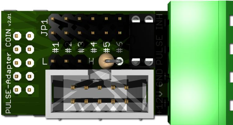
The [PULSE-Adapter COIN](#) has a 10 pin connector that fits to default coin plugs, and offers again a 10 pin coin plug to plug in the originally coin acceptor cable, so you do not lose the coin acceptor connector.
