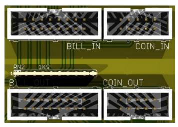
To test a 10 pin cable plug it into the COIN IN and COIN OUT connector.
