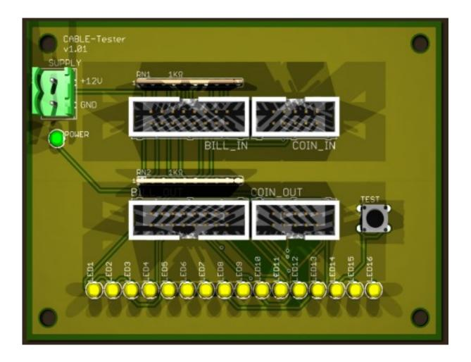
Each wire (1-10 or 1-16) is assigned an LED and it is tested separately. The LEDs 1-10 are used for the 10 pin cable, 1-16 for the 16 pin cable.
