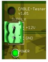
The CABLE-Tester can work with a voltage range of 5-24 Volt DC. Connect power supply to the SUPPLY connector.
