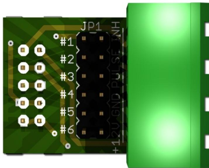
Nayax and OTI pulse connection it is just power (plus and minus) and the pulse signal.
