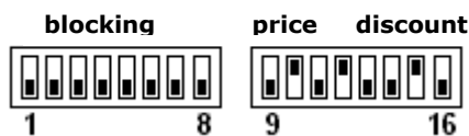
Fig. 19 Assignment of the DIP switches when the price setting is programmed to be carried out via DIP switches
