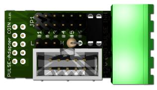
The **PULSE-Adapter COIN** has a 10 pin connector that fits to default coin plugs, and offers again a 10 pin coin plug to plug in the originally coin acceptor cable, so you do not lose the coin acceptor connector. The cashless device can be connected easily via plugable terminal connector. With a jumper you can select the coin channel on which the external credit signal is transferred. Additionally there is
